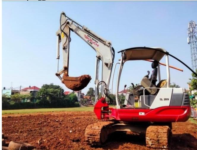
Gambar 2. Unit *Mini Excavator* TB260 Takeuchi
