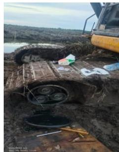
Gambar 3 5 Pembongkaran Housing Planetary Gear
