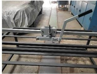
Gambar 6. Jig Sliding Cutting
