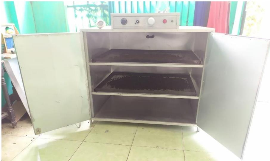
**Gambar 2.** Alat Pengering Biopellet.
