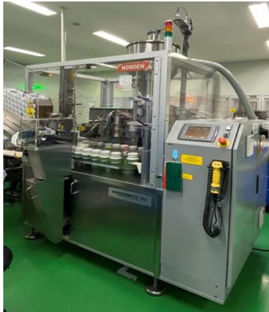
*Gambar 2.1 Mesin Filling Up Tube Nordenmatic 702*
