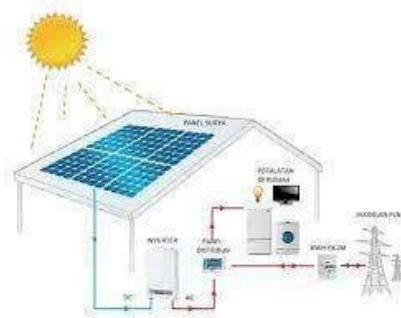
Gambar 5 Sistem PLTS On – Grid
