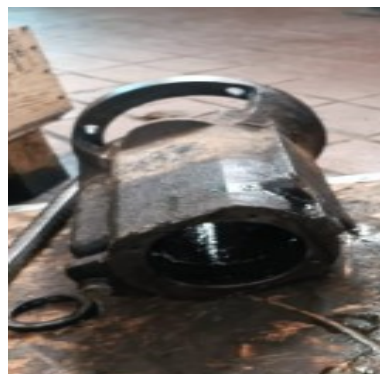
Gambar 3. 2 Kondisi Housing Bearing Kotor
