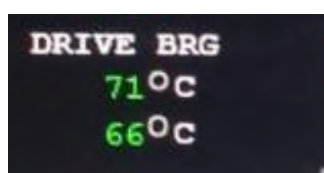
Gambar 2. Pemantauan Temperature Drive Bearing Gear Symetro 564-MD1
