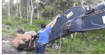
Gambar 9 Remove Cylinder Bucket
