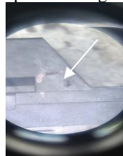
Gambar 3. 3 Sampel cacat short mold scoring
