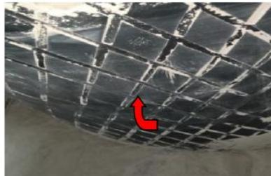
Gambar 10. Pengecekan Legging Pulley
