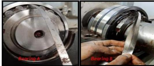
Gambar 9. Pengukuran Bearing Head Pulley
